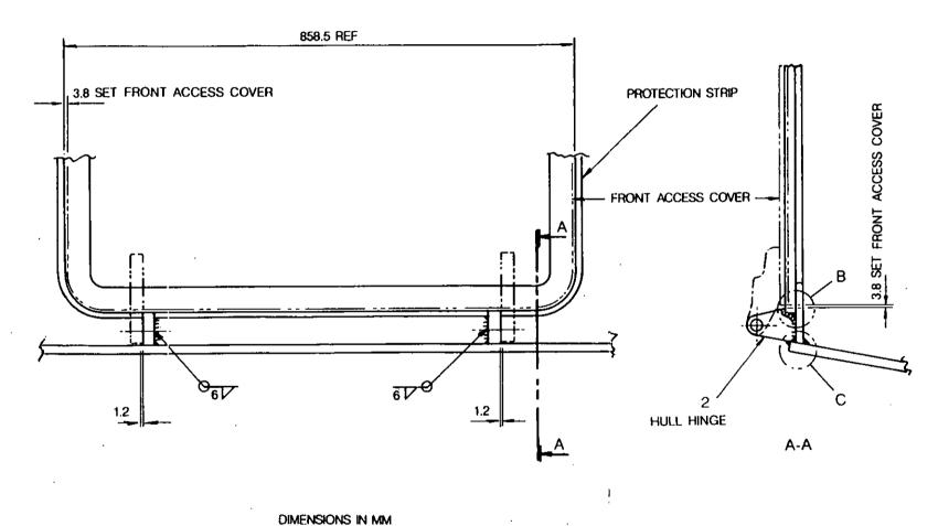
Fig 2 Replacement of the front access cover hinges (hull), set from the hatch hinges
